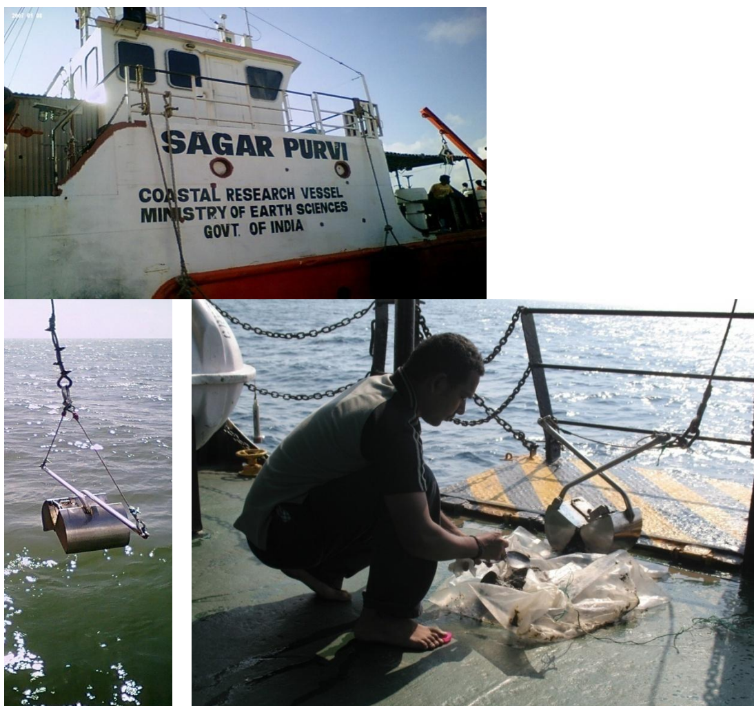
Plate 1: Collection of surface sediment samples by using Van Veen Grab sampler in the inner shelf of Adyar River Mouth Traverses of Bay of Bengal
