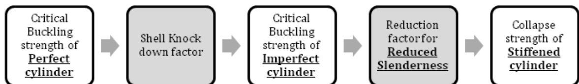
Figure 1: Elements of a typical analytical strength model of stiffened cylinder
